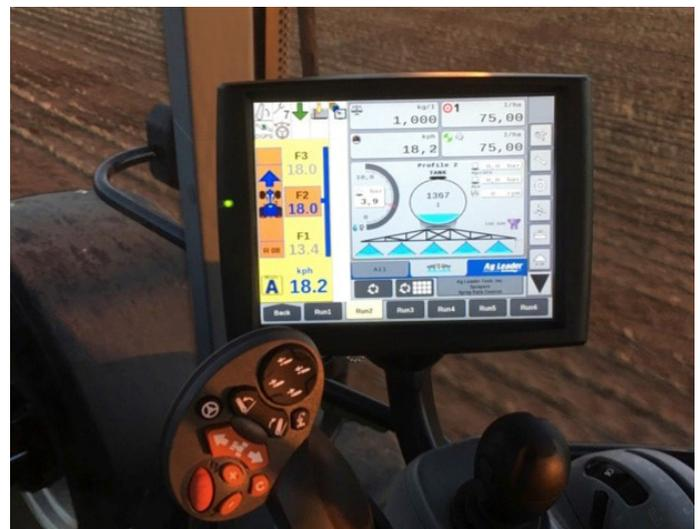
Above - Spraying monitor with auto section in operation
